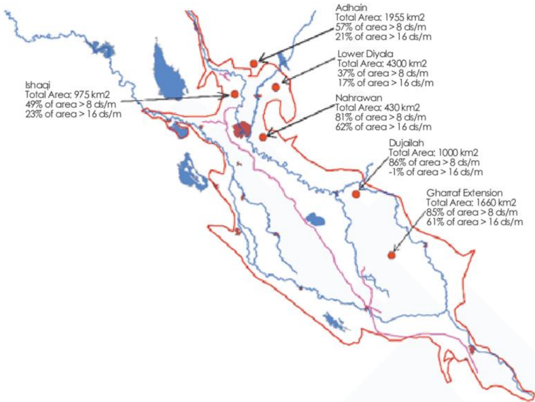
Figure 37. Location of projects with indication of saline areas in the Mesopotamian plain (Moutaz, 2013)
