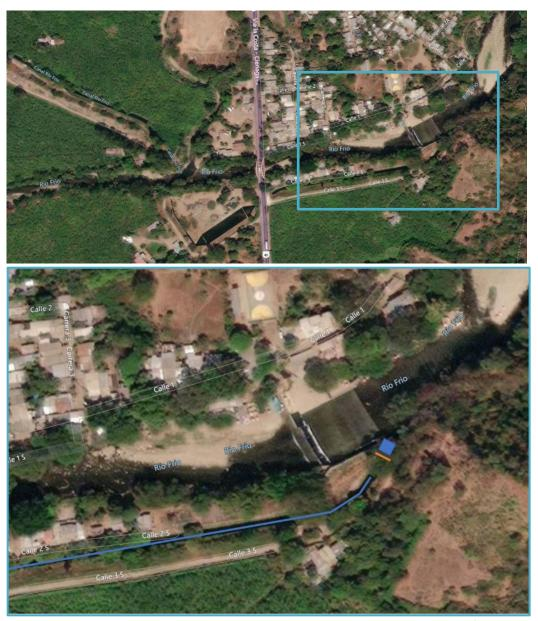
Figure 4-3. The Río Frío, at the village Río Frío, and the primary water infrastructures of ASORÍOFRIO, with the main intake (blue square), the weir structure (orange line), and canal Santa Inés (blue line), in zoom below, Bing maps Imagery.
