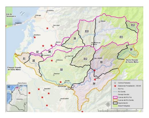
Figure 5-3: Numbered sub-catchments / river segments and precipitation stations in the Río Frío and Río Sevilla catchments in Magdalena Province as used for the Environmental flow assessment. Source WWF Colombia and CORPAMAG (2020).
