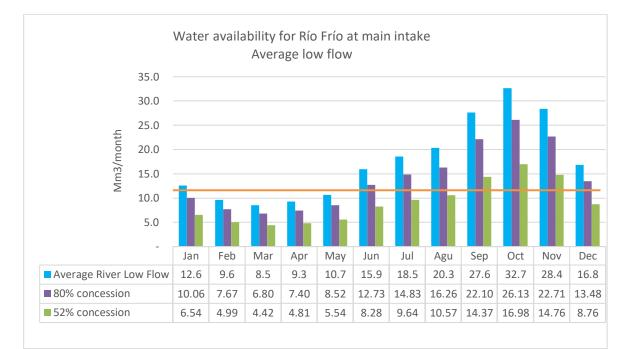
Figure 6-4: The figure shows the lowest average (median) monthly river flow over the years 1965 – 2015 for Rio Frío with the corresponding dynamic concessions of 80% intake or 52% intake for ASORIOFRIO. Orange line indicating the maximum intake of ASORIOFRIO of 12.71 Mm3/ month based on the concessions for ASORIOFRIO and the private concessions combined.
