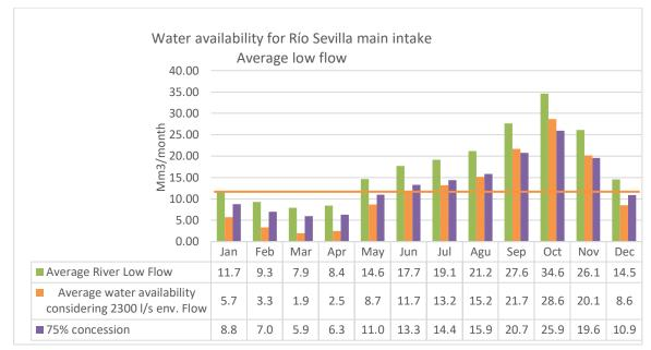
Figure 6-6: The figure shows the lowest average (median) monthly river flow over the years 1965 – 2015 for Rio Sevilla with the corresponding dynamic concessions of 75% intake fixed environmental flow of 2300 I/s for ASOSEVILLA. Orange line indicating the maximum intake of ASOSEVILLA of 11.42 Mm3/ month.
