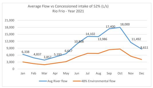
Figure 6-2: Monitored intake data of ASORIOFRIO confirms that for 2021 a dynamic environmental flow of 48% (Intake of 52%) was considered, instead of 20% environmental flow or a fixed environmental flow.
