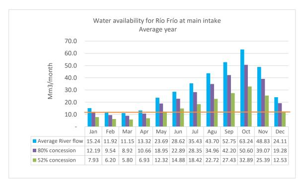
Figure 6-3: The figure shows the average (Q50, median) river flow over the years 1965 – 2015 for Rio Frío, with the corresponding dynamic concessions of 80% intake or 52% intake for ASORIOFRIO. Orange line indicating the maximum intake of ASORIOFRIO of 12.71 Mm3/ month based on the concessions for ASORIOFRIO and the private concessions combined.
