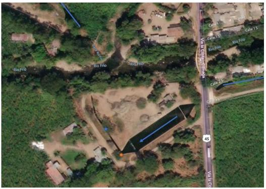
Figure 4-4. The Río Frío, at the village Río Frío, and the hydrological monitoring station of the ASORIOFRIO intake (blue dot), main channel (known as Santa Inés, blue line on the right) and intake of the private concession (orange dot) at ASORIOFRIO. Bing Maps Imagery.
