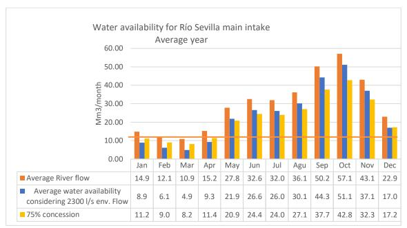
Figure 6-5: The figure shows the average (Q50, median) river flow over the years 1965 – 2015 for Rio Sevilla with the corresponding dynamic concessions of 75% intake fixed environmental flow of 2300 I/s for ASOSEVILLA. Orange line indicating the maximum intake of ASOSEVILLA of 11.42 Mm3/ month.
