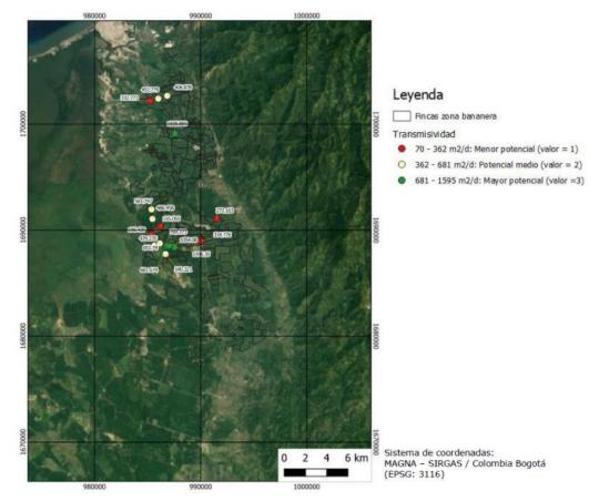
Figure 2-4 This map shows the available transmissivity values (in m<sup>2</sup>/d). These vary spatially, not observing any specific trend. This gives indication of the high heterogeneity of the aquifer. Source: RECARBA project, Deltares (2021b).
