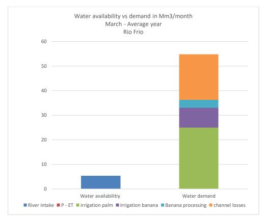
Figure 6-7 Theoretical water balance for the Río Frío for the month of March for an average year. 48% environmental flow is considered to calculate the water availability. The water demand was calculated to provide all crops with an optimal yield.
