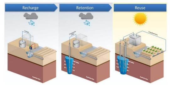
Figure 50. An example of an Aquifer Storage and Recovery(ASR) system. Image of Acacia Water.
