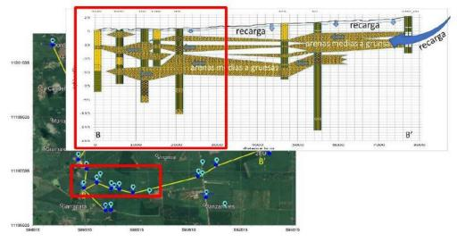
Figure 2-5. This figure indicates the field information for the Don Said farm based on well information. In this zone, the depth at the static level is between 3.3 m to 12.8 m, while the electrical conductivity varies between 79 to 753 µS/cm. Expected recharge flows are indicated in the figure. Source: RECARBA project, Deltares (2021b).
