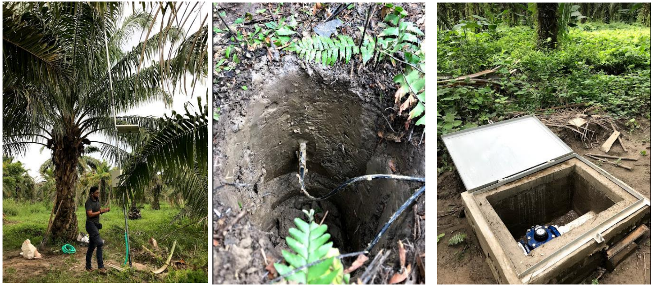
Figure 5. Establishment of the pilot study. Left and middle: establishment of soil moisture content sensor. Right: establishment of water meter.
