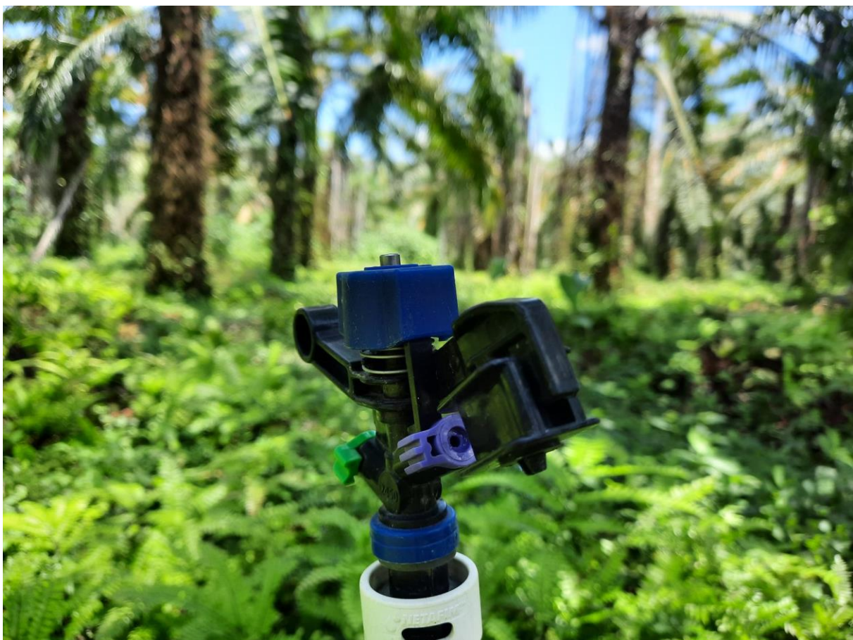
Figure 3. Sprinkler irrigation system, impact type.
