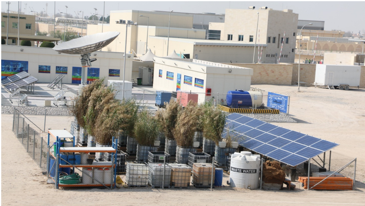
Research set-up in the Middle East (Shell): Energy by solar panels to pump water through containers with plants to purify waste water
